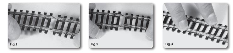
**NOTE :-** If assembled track must be moved, care should be taken to avoid bending the track where sections connect. It is always best to assemble the track where it is to be operated.
