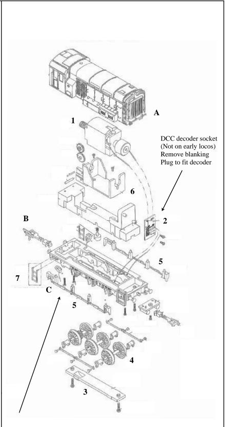
Body removal - Release the wire from the footplate front near "A". Remove rear coupling pocket B. Remove single screw "C" and release body clip adjacent. Cab and bonnet assembly will then pivot forwards to lift clear of the footplate.
