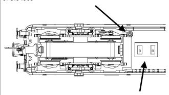
Switches for cab lights and tail lights on/off
