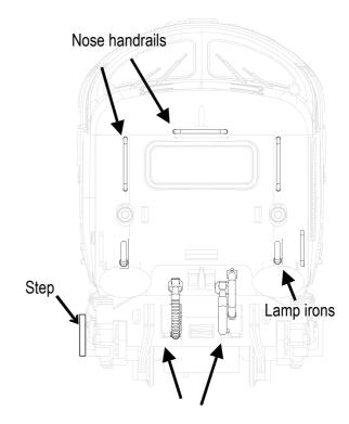
Brake and heating pipes
