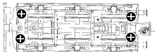
Tender shell secured by screws at corners
