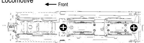
Loco chassis secured by screws at outside of driving wheels
