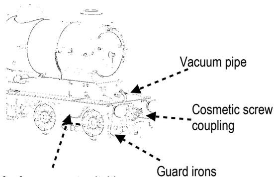
Fillets for frames - not suitable when run on tight radius curves
