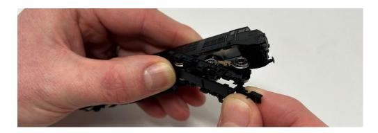
3. With the bogie frame removed, it can be seen that the middle 'mound' (red arrow) moulded onto the bottom of the bogie frame is deeper than those at either end (green arrows). Gently file the middle mound to the same height as the other two and this should resolve the grounding issues that some users are experiencing when running on Code 55 'finescale' Points & Crossings.
