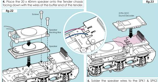
**5.** Place Speaker Backing Box over the speaker with the wires passing through the opening. Secure in place using the two screws that are packed with the accessories.
