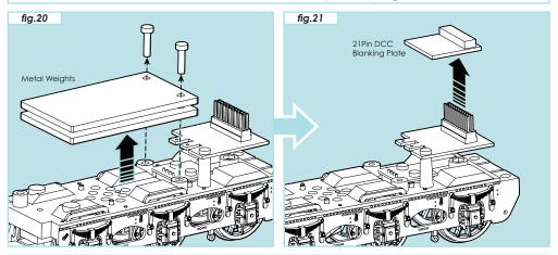
3. Remove the metal weights, held in by two screws, and the 21 Pin DCC blanking plate.
