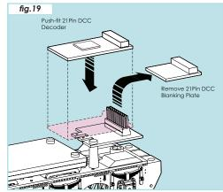
**3.** Remove the 21 Pin DCC blanking plate and pushfit the 21 Pin DCC decoder onto the pins of the PCB as shown.
