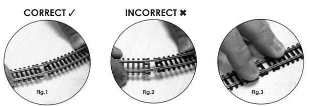
**NOTE :-** If assembled track must be moved, care should be taken to avoid bending the track where sections connect. It is always best to assemble the track where it is to be operated.
