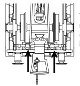
Tender securing screw located under coupling pocket (secured by the two screws indicated)
