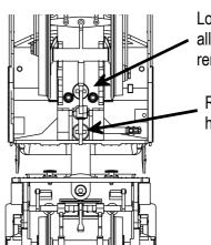
Loosen this screw to allow the drawbar to be removed from chassis
