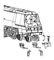
Carefully remove the blanking board above the motor and replace with a decoder having a NMRA/NEM 651 6-pin fitting.
