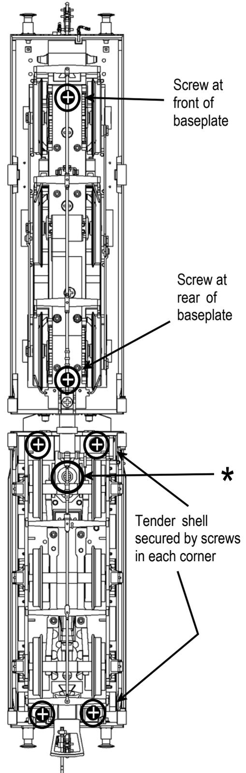
\* Adjustable length tender draw bar is secured by the screw indicated - slacken a little to allow bar to slide
