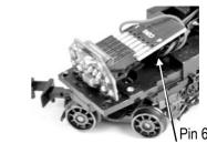
Location / alignment of blanking plug or decoder
