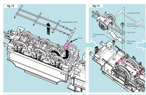
1. Remove the Brake Gear then disconnect the plug from the underside of the Tender. The Tender can now be removed.
