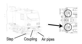
The plough fitted can be removed should it be desired to fit functional couplers to the unit - remove the two screws indicated
