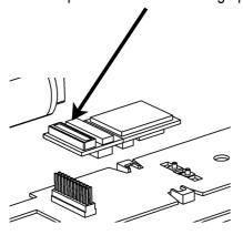
structions included with the decoder: the decoder fits so that the contact block is uppermost.
