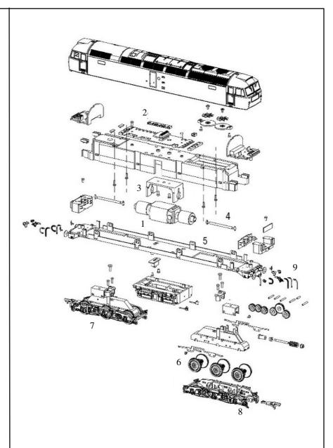
Location and alignment of 21-pin DCC decoder
